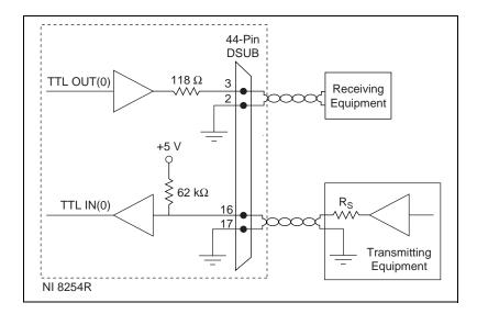
When connecting to TTL inputs on the NI 8254R, match the output impedance of the transmitting device to the characteristic impedance of the cable. For example, if the cable characteristic impedance is 118  $\Omega$ , make  $R_s$  equal to 118  $\Omega$ , as shown in the figure above.
